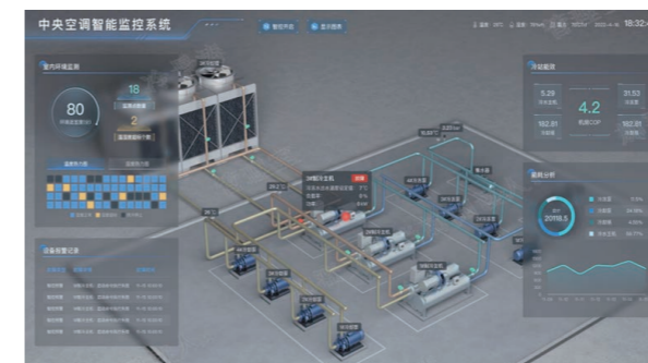
Central Air Conditioning Intelligent Monitoring System
